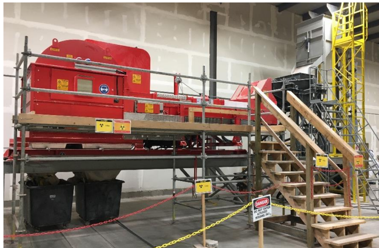
Fig. 4 TOMRA COM Tertiary XRT Ore Sorter used in the ore sorting Performance Test at SRC
