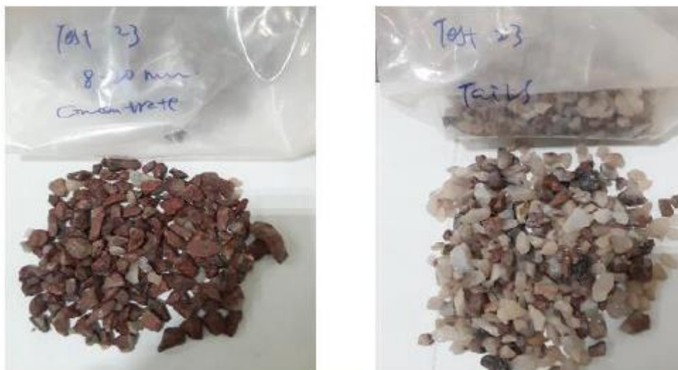
Figure 1 A product and corresponding reject sample from one of the sorter runs. Red is high grade (>50% REO) bastnasite concentrate with white being waste (quartz) material.
