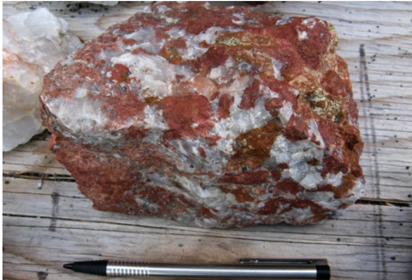
Fig. 3: Ore sample from North T Zone showing red bastnaesite crystals with quartz waste
