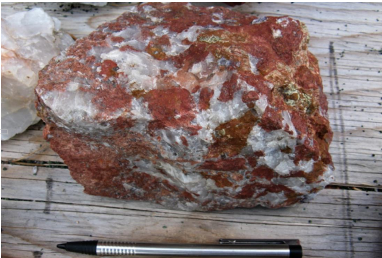
Fig 3: A sample of North T mineralised ore. Rare earths are contained within the red bastnaesite minerals and white material is quartz waste rock. Vital intends to initially separate the bastnaesite materials via conventional ore sorting technology.
